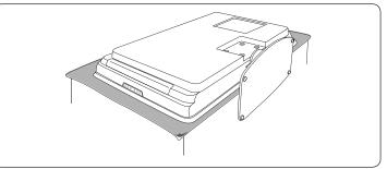
2. Using a cross-head (Phillips) screwdriver (not supplied), unscrew the four screws that secure the stand to the TV.
